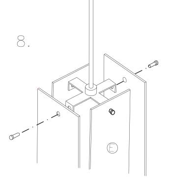
Attach the 2 wide (3" wide) glass pannels **Pannel should hang freely, do not over-tighten** Make sure the glossy side is facing outwards
